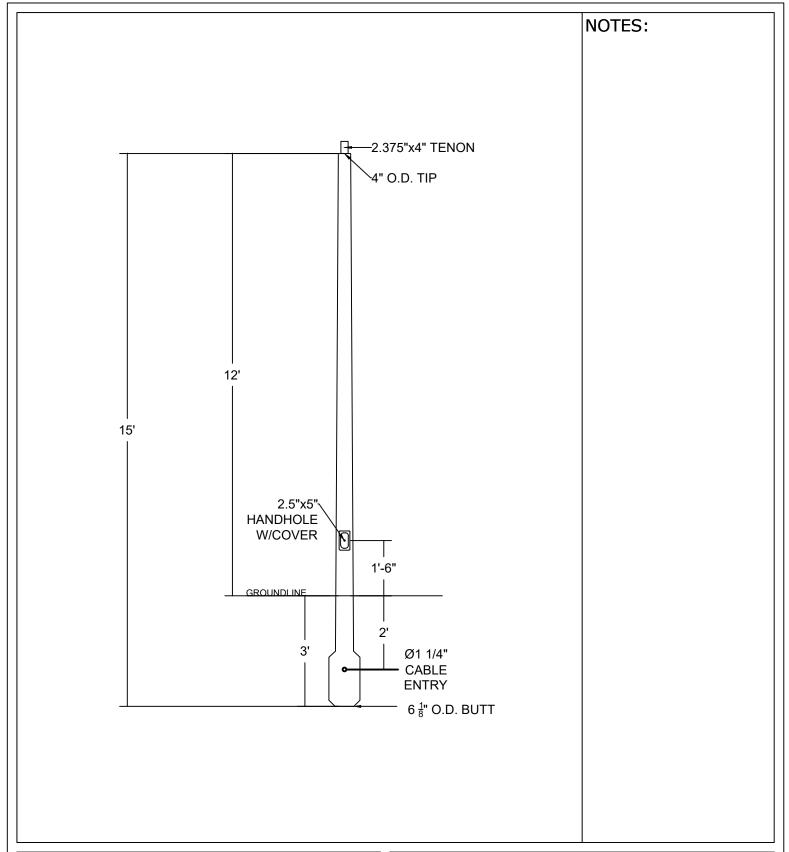
FILAMENT WOUND SECTIONAL COMPOSITE SHAFT CONSISTING OF CONTINUOUS FIBERGLASS ROVING COMBINED WITH THERMOSETTING POLYESTER RESIN WOUND IN LOW ANGLE HELIACAL AND HIGH ANGLE HOOPS PROVIDING FOR MAXIMUM RESISTANCE TO DEFLECTION AND SHEAR. POLE FINISH IS A 10-15 ML THICK POLYESTER FINISHING RESIN. DIRECT BURIAL POLE ASTM 4923 CLASS 1 (POLE TOP DEFLECTION SHALL NOT EXCEED 15% OF THE ABOVE HEIGHT @ MAX WIND LOADING AND MAX FIXTURE WEIGHT) DESIGN CRITERIA PER 2017 FBC 6TH EDITION AND ANSI C136.20-2012
