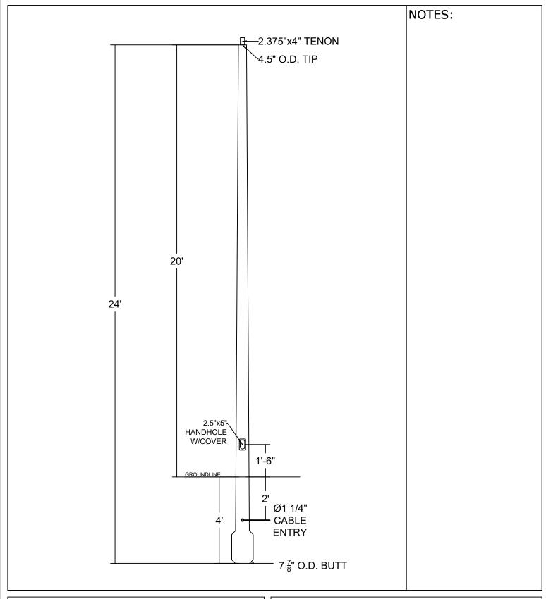
FILAMENT WOUND SECTIONAL COMPOSITE SHAFT CONSISTING OF CONTINUOUS FIBERGLASS ROVING COMBINED WITH THERMOSETTING POLYESTER RESIN WOUND IN LOW ANGLE HELICAL AND HIGH ANGLE HOOPS PROVIDING FOR MAXIMUM RESISTANCE TO DEFLECTION AND SHEAR. POLE FINISH IS A 10-15 ML THICK POLYESTER FINISHING RESIN. DIRECT BURIAL POLE ASTM 4923 CLASS 1 (POLE TOP DEFLECTION SHALL NOT EXCEED 15% OF THE ABOVE HEIGHT @ MAX WIND LOADING AND MAX FIXTURE WEIGHT) DESIGN CRITERIA PER 2017 FBC 6TH EDITION AND ANSI C136.20-2012
